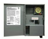
Each unit includes a UL Approved Control Panel complete with Class A Human Rated GFCI Protection, 24 Hour Mechanical Timer, and Photo Eye for Optional Light Kit. NEMA Type 3R weatherproof enclosure. 5.1VFX must be hardwired into control panel.
