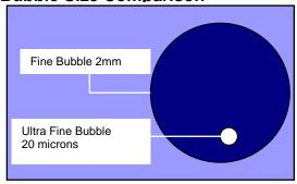
bubbles stay resident in the water for up to 10 minutes and the dissolved oxygen can remain for 4-6 hours.
