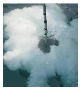
Microbubble Turbine Technology is a self-aspirating aerator. This means that it draws air by suction from the atmosphere. It does not need high-dollar canister oxygen or a compressed air system to generate and inject oxygen into the body of water. Also, due to its design, it is virtually impossible for the turbine to clog.
